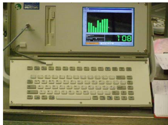
Figure 7: Measuring station for the gamma sensor
